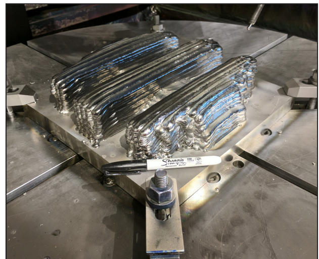
Figure 1: Small sample part built using the electron beam additive manufacturing process.
