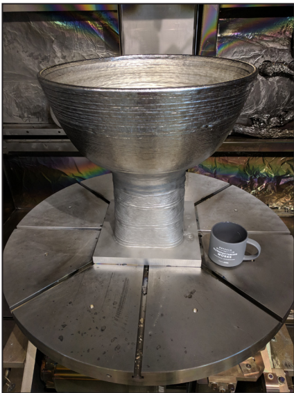
Figure 2: Large sample part built using the electron beam additive manufacturing process.
