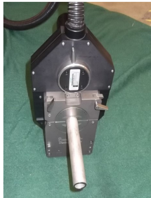
Figure 2: 1/2 in. Schedule 40 Pipe Specimen Positioned in a Closed-Frame Orbital Welding Head
