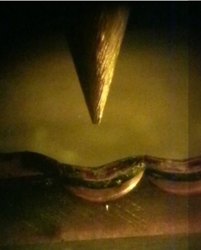
Magnified photo of edge welds on copper
