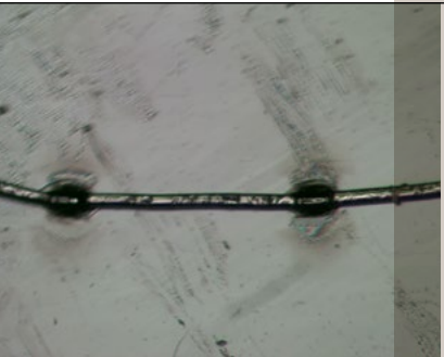
Platinum wire parallel-gap welded to a titanium film on glass
