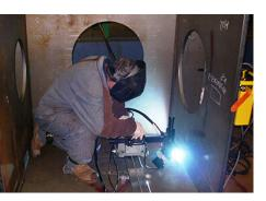
EWI was able to increase the deposition rate and use less filler material while maintaining the required heat input. This allowed a 33% increase in overall productivity while meeting all mechanical property requirements.
